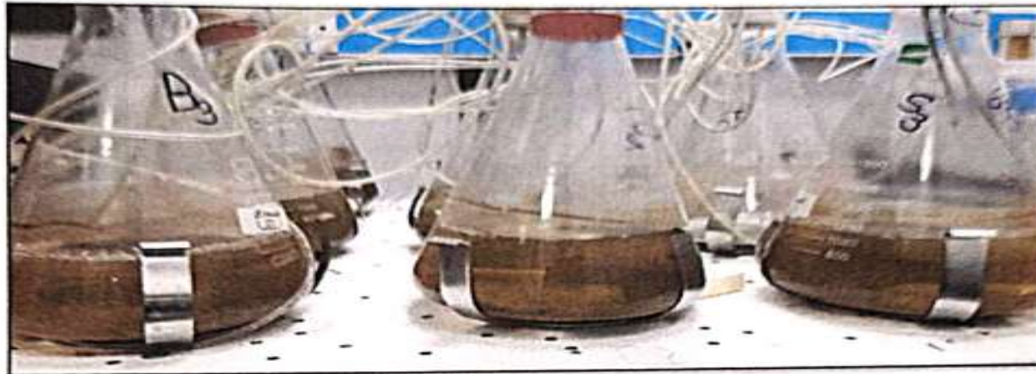
Figure 2. Test setup for Biodegradation of test and reference substances in replicates
